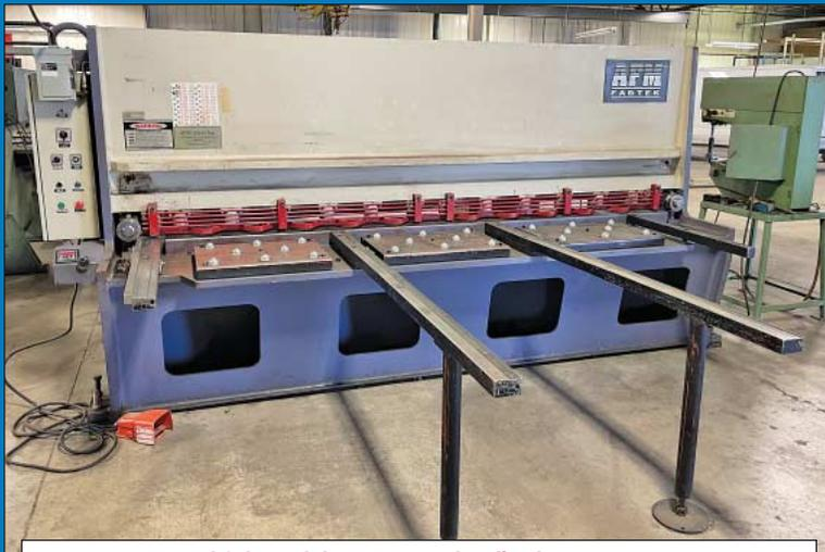
1/4" x 10' AFM Fabtek Model MK 6-31 Hydraulic Shear
