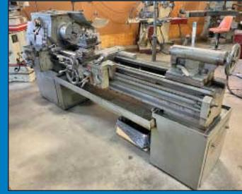
16" x 30" American Pacemaker Engine Lathe with Taper Attachment
