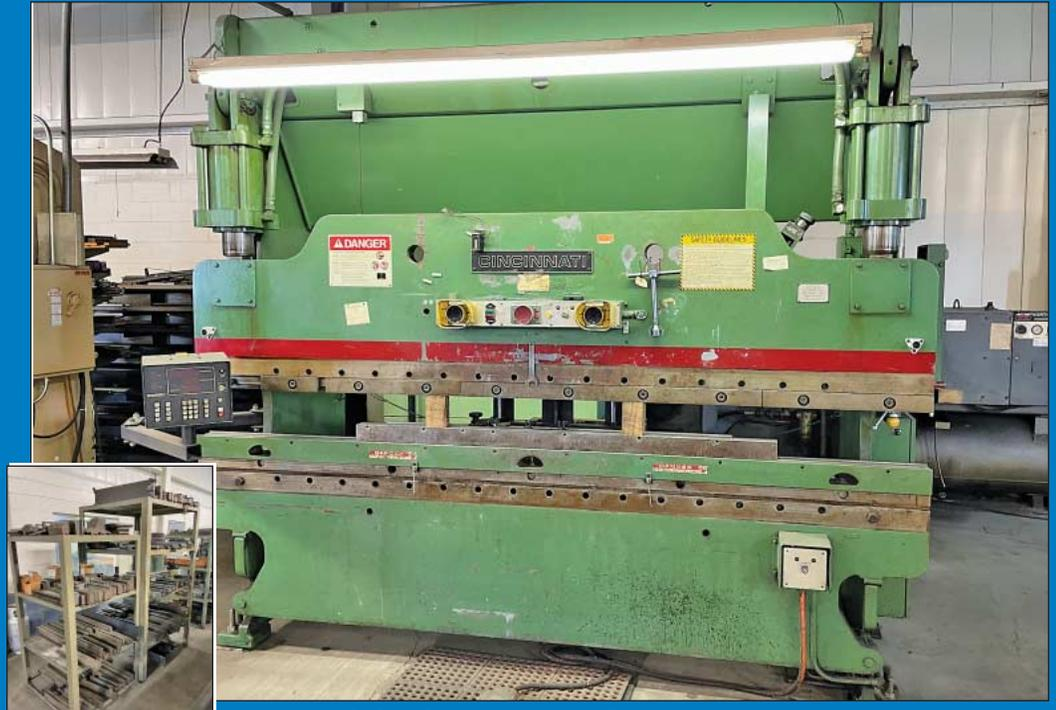
90 Ton x 10' Cincinnati Model 90CB Hydraulic Press Brake
