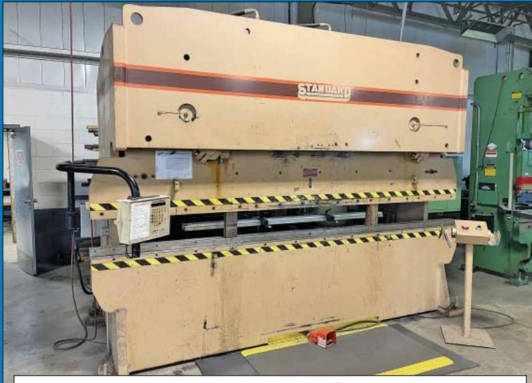
200 Ton x 12' Standard Model AB200-12 Hydraulic Press Brake
